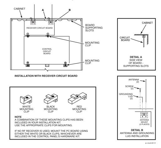
Figure 3. Mounting the PC Board and RF Receiver
